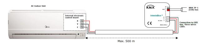
IntesisBox<sup>®</sup> MD-AC-KNX-1B/16/64 allows monitoring and control, fully bi-directionally, of all the functioning parameters of Midea Air Conditioners from KNX installations.
